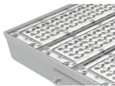
Lens PC lens, light transmittance >90%, Flammability rating: UL94-V0; 30°, 60°×90° beam angle optional.
